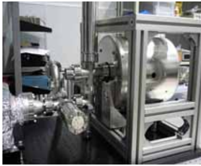
Figure 8. The two-layer magnetic shield for ion trap of ^{40}\text{Ca}^+ ions. In the magnetic shield (right side), there are a vacuum chamber (70-mm cube) and three pairs of magnetic coils.
